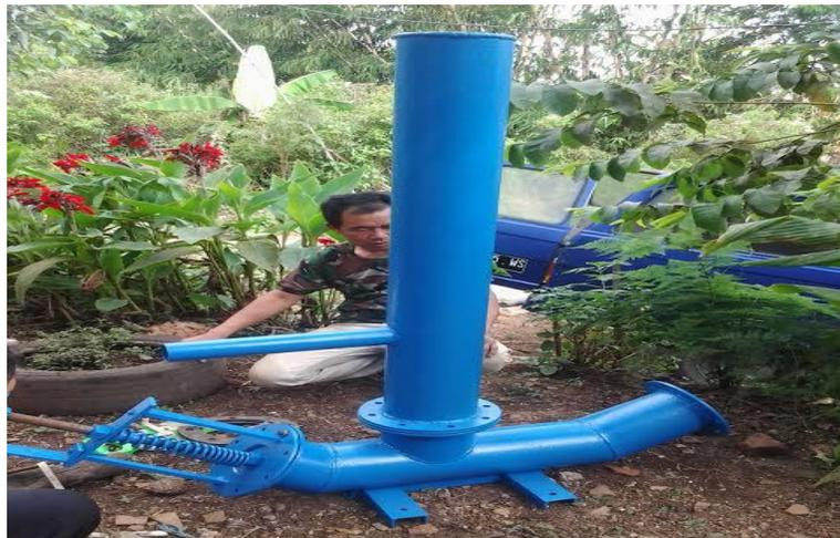
**Gambar 2.2** Pompa Hydraulic Ram
